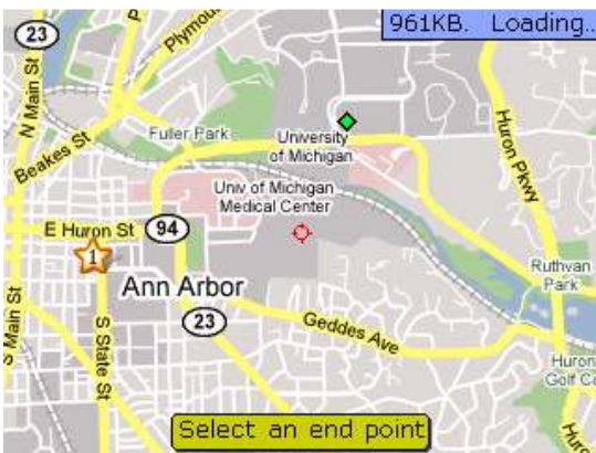
Figure 13: The data transfer feedback box only displays how much data has been loaded, not what portion of the total data to be loaded.
